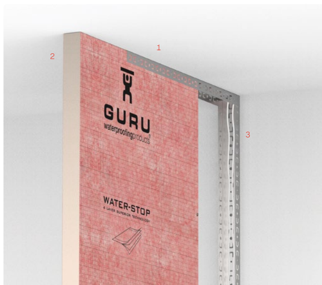
1. Perfil de montagem / 2. W-S Board (2600 × 625 × 50 mm) / 3. W-S Mastic
