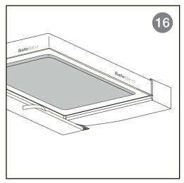
Now start to peel the narrow flange (see image 15) and stick it on the flank and on adjacent side band (see image 16). Once the entire strip is attached, press hard with the squeegee shovel all the way around. Trim the excess.
