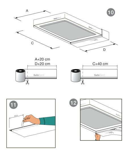
The band in the sides facing to floor shall turn up in the walls and be connected to the band of the other sides. Remove the widest release paper about 20 cm (8") (see image 11) and start sticking from a corner on the underside of the shower tray or bathtub (see image 12). The narrow flange, still with its release paper, should stand on the flank.
