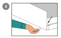
Remove some more release paper and carry on sticking keeping the straight line. Before bend at the corners, make a small cut in the narrow flange to facilitate folding (see image 5).
