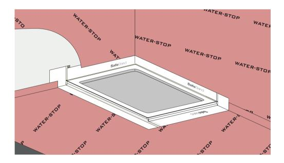
Once the shower tray or bathtub is installed in its final position, proceed to stick **Safe**Band to the walls and floor with C2 class tile adhesive. Install waterproofing in floors and walls if planned. **Safe**Band must be overlapped by the walls membrane while overlapping the membrane at floor.
